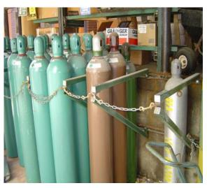
Cylinders, valves, regulators, hoses as well as other apparatus and fittings for oxygen shall be kept free from oil and grease. Oxygen cylinders, apparatus, and fittings shall not be handled with oily hands, oily gloves, greasy tools or equipment.
